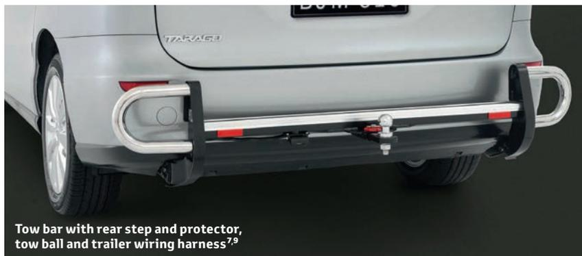
Tow bar with rear step and protector, tow ball and trailer wiring harness<sup>7,9</sup>
